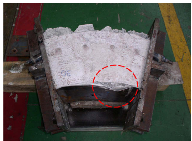
Fig. 14. Buckled steel plate of D200H75T2.
